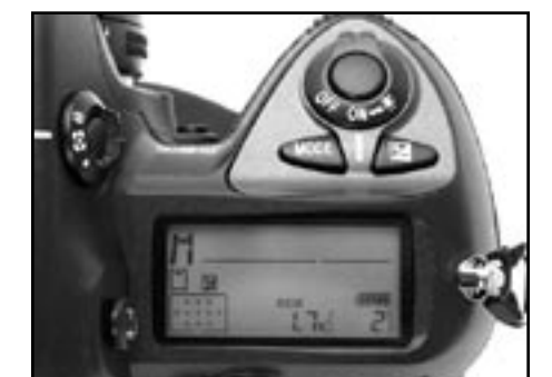
Nikon has expanded the top panel LCD display since the D1 series. The D2H can fire off eight shots per second into a 40-second buffer.
