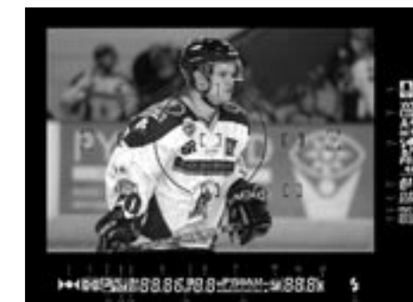
Nikon has expanded the amount of information provided in the viewfinder display; it now also includes 11 autofocus areas, white balance setting, ISO and image size/quality.
