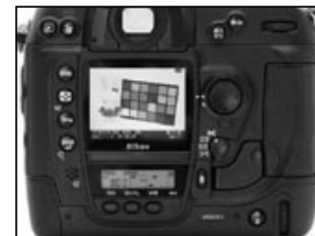
The D2H has an extra large 2.5 inch LCD monitor with a 211,000 pixel resolution. The real panel is better organized to accomplish functions faster.
